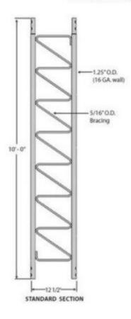
The 25G antenna tower is a light weight tubular tower with solid braces. The tower sections can be guyed, but can also be used in bracketed and self-supporting applications. Standard sections are 10' in length.
